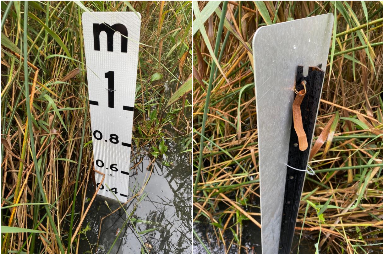
Photo 1 Water measuring gauge
